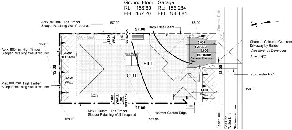
All Required Fencing to be Timber Rail & Paling 1800H with access gates as shown.
